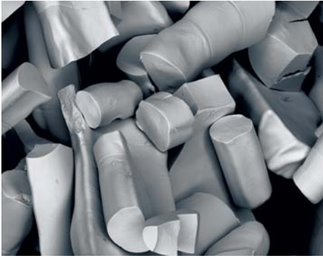
Fig.: High resolution SEM micrograph of Ni-Mn-Ga fibres to be embedded into a polymer matrix.
