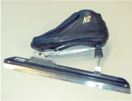
Fig.: New skating blades made of nickel-based super-alloy <040S> embedded in a carbon fibre runner of the K2 speed skating shoe [made available by FES Berlin].
