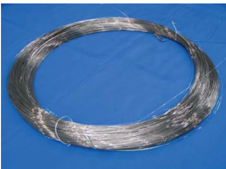
Fig.: First 1000 m multifilamentary MgB 2 wire using mechanically alloyed in-situ powder manufactured under industrial production conditions
