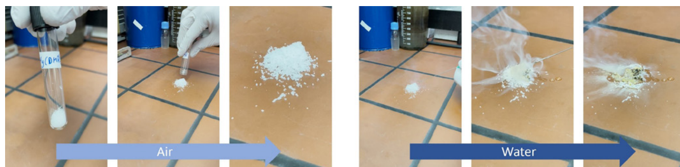
Fig. 3: Image series captured from a video showing the exposure of about 500 mg of pristine [\text{Mg}(\text{DMP})_2] to air for approximately two minutes, followed by reaction with \text{H}_2\text{O} .
