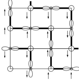
Figure 1.3. Charge, orbital and spin ordering in the basal ( $xy$ )-plane of manganates at  $x = 0.5$ . Arrows denote the spin ordering. The spin zigzags, typical for the CE-type magnetic order, are shown by thick lines.
