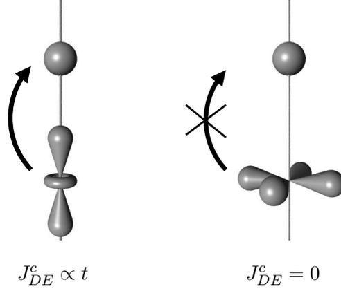
Figure 1.11. The  $e_g$ -electron transfer amplitude, which controls the double-exchange interaction  $J_{DE}$ , strongly depends on the orbital orientation: along the  $z$  direction, e.g.,  $d_{3z^2-r^2}$  electrons (left) can hop into empty sites denoted by a sphere, while the transfer of  $d_{x^2-y^2}$  electrons (right) is forbidden [86].
