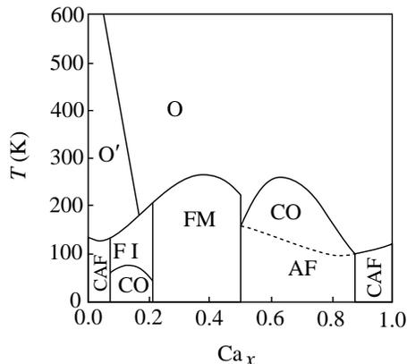
Figure 1.1. Phase diagram of  $\text{La}_{1-x}\text{Ca}_x\text{MnO}_3$  (after S.-W. Cheong). O: orthorhombic phase with rotated regular octahedra, O': orthorhombic phase with Jahn-Teller distortions, CAF: canted antiferromagnet or phase separated state, FI: ferromagnetic insulator, CO: charge order, FM: ferromagnetic metal, AF: antiferromagnet.
