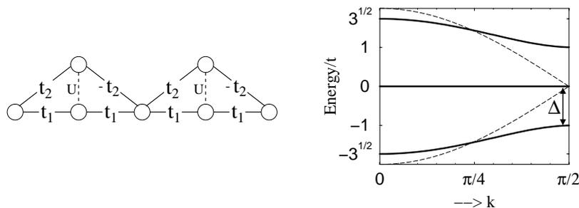
Figure 1.13. Left: Topology of the interactions in a zig-zag chain, where  $t_1 = t/2$ ,  $t_2 = t\sqrt{3}/2$ , and  $U$  is the Coulomb interaction between electrons on the same site. Right: electron dispersion in the zig-zag chain of the CE-phase for  $U = 0$  (solid lines) and electron dispersion in a straight chain, as in C-phase (dashed lines).
