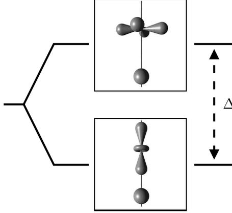
Figure 1.9. Polarization of  $e_g$ -levels on sites next to a hole [51]: Bond stretching phonons and Coulomb interaction induce a splitting of energy  $\Delta = \Delta^{\text{ph}} + \Delta^{\text{ch}}$ . Here the sphere indicates the location of a hole ( $\text{Mn}^{4+}$ -ion) adjacent to a  $\text{Mn}^{3+}$ -ion.
