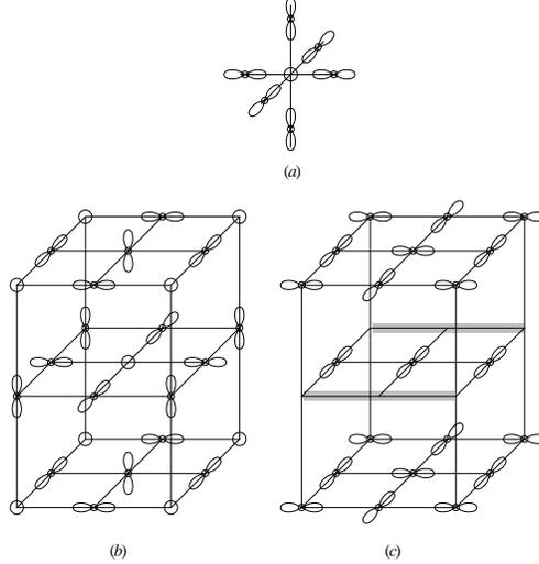
*Figure 1.5.* Orbital polarons and possible types of orbital ordering in low doped manganites: (a) Orbital polaron close to a  $\text{Mn}^{4+}$  ion; (b) Ordering of orbital polarons for  $x = 0.25$  in a bcc-lattice; (c) An alternative charge and orbital ordering, obtained for  $x = 1/8$  in [34]. Notations are the same as in Figs. 1.3 and 1.14. Shaded lines–“stripes” containing holes.
