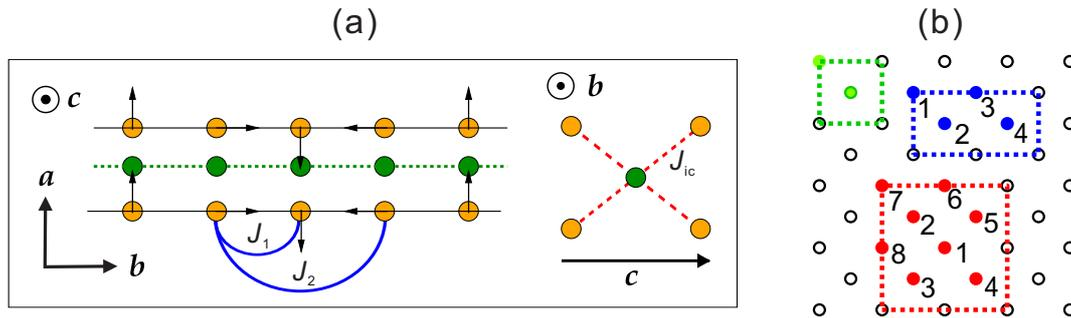
**Figure 1.** (a) Lattice structure of the coupled frustrated Heisenberg chains. (b) The 3D arrangement of chains used for the DMRG calculation.
