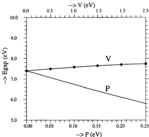
Fig. 2. Value of the conduction gap  $E_{\text{gap}}$  as a function of the inter-site Coulomb repulsion  $V$  and polarization screening  $P$ , for a two-dimensional eight-site extended Mott–Hubbard cluster. Upper curve with dots:  $V$  is varied between 0 and 2.5 eV. Lower curve:  $P$  is varied between 0 and 0.25 eV. The bare Coulomb repulsion  $U_0$  is kept constant at 10 eV. The hybridization  $t$  is 1 eV.
