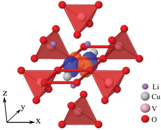
FIG. 2. (Color online) Chain of edge-sharing  $\text{CuO}_4$  plaquettes in  $\text{LiVCuO}_4$ . The ground-state hole orbital is  $d_{xy}$  in the chosen reference system. The six NN  $\text{VO}_4$  octahedra around the reference Cu site are highlighted in the figure.
