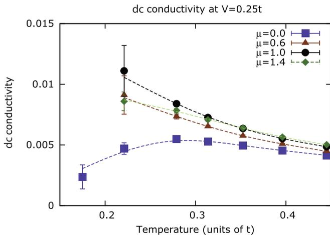
FIG. 11. (Color online) The dc conductivity  $\sigma_{dc}$  following Eqs. (30) and (31) at  $V = 0.25t$  as a function of temperature for different doping levels, with for  $N_x = 6$ . The temperature dependence of the conductivity indicates that the undoped  $\mu = 0$  state is indeed insulating, while  $\mu = 1.0$  shows metallic behavior. We have set  $U = 4t$  and  $t_{\perp} = 0.05t$ .
