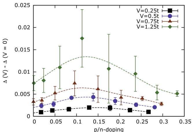
FIG. 8. (Color online) Interlayer tunneling for  $N_x = 6$  at  $T = 0.221t$ ,  $U = 4t$ , and  $t_{\perp} = 0.05t$ , relative to the  $V = 0$  case, for all densities and interaction  $V$ . A clear enhancement of the tunneling, which is equal to the exciton condensate order parameter, can be seen around the doping level of 10–20%.
