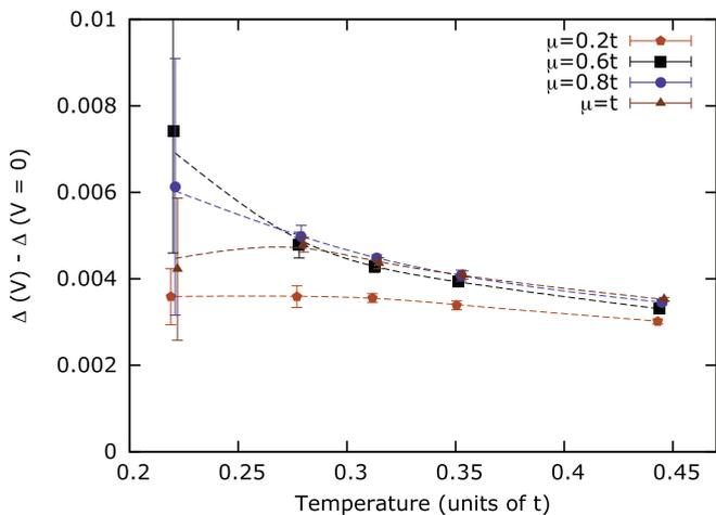
FIG. 7. (Color online) Interlayer tunneling at  $V = 0.75t$ ,  $U = 4t$ , and  $t_{\perp} = 0.05t$  for  $N_x = 6$ , relative to the  $V = 0$  case. A clear enhancement of the tunneling amplitude, which is equal to the order parameter of the exciton condensate, can be seen around  $\mu = 0.8t$ , where the doping level is approximately 15%.
