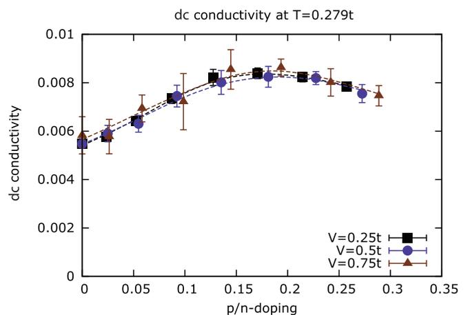
FIG. 10. (Color online) The dc conductivity  $\sigma_{dc}$  following Eqs. (30) and (31) at  $T = 0.279t$  as a function of doping and  $V$  for  $N_x = 6$ . The dc conductivity is the largest at a doping around 15–20%. We have set  $U = 4t$  and  $t_{\perp} = 0.05t$ .
