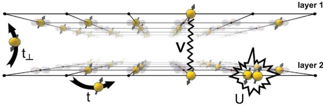
FIG. 1. (Color online) The extended bilayer Hubbard model, Eqs. (1)–(4), describes two layers with in-plane hopping  $t$  and interlayer  $t_{\perp}$ , on-site repulsion  $U$ , and interlayer Coulomb interaction  $V$ . In this paper we study this model using DQMC.
