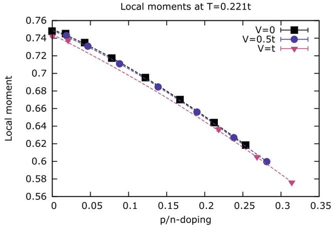
FIG. 14. (Color online) The local moments as a function of  $V$  and doping at  $T = 0.221t$  for  $N_x = 6$ . The localization of electrons is the strongest at half filling, and almost independent of the interlayer interaction  $V$ . We have set  $U = 4t$  and  $t_{\perp} = 0.05t$ .
