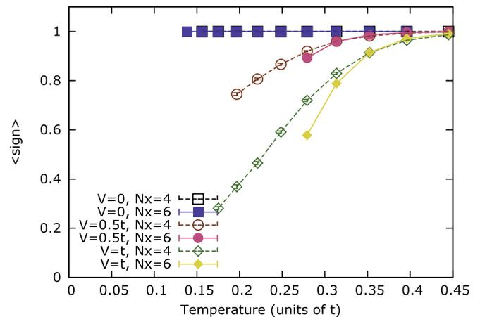
FIG. 3. (Color online) The average sign at half filling for various interlayer interactions  $V$ . When  $V \neq 0$  the average sign drops rapidly. Parameters are  $U = 4t$ ,  $t_{\perp} = 0.05t$ , and  $\mu = 0$ .
