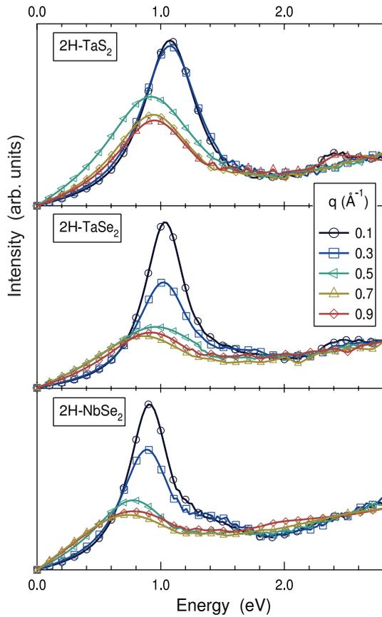
FIG. 1 (color online). The EELS intensity for the three investigated compounds measured at room temperature. The spectra have been normalized on the high-energy side and the data for  $2H\text{-TaSe}_2$  are partially reproduced from Ref. [17].
