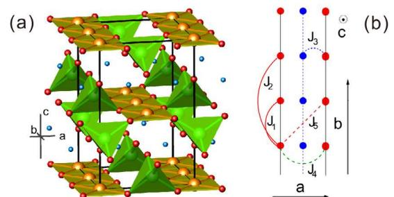
Fig. 1: (a) The crystallographic structure of  $\text{LiVCuO}_4$  with two  $\text{CuO}_2$  chains per unit cell running along the  $b$ -axis (orange dots:  $\text{Cu}^{2+}$ , red dots:  $\text{O}^{2-}$ , bright blue dots:  $\text{Li}^+$ ). (b) The main in- and inter-chain exchange paths,  $J_1$ ,  $J_2$ , and  $J_3$ ,  $J_4$ ,  $J_5$  marked by red solid arcs, broken line, blue and green arcs, respectively.
