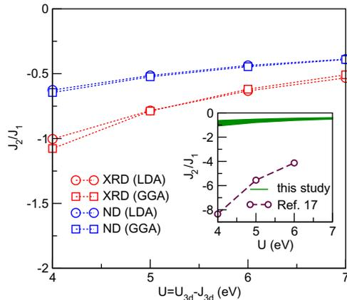
Fig. 7: Frustration parameter  $\alpha$  vs. effective on-site repulsion  $U$  for different crystal structure refinements from X-ray (XRD) and neutron diffraction (ND). Inset: the obtained  $\alpha$ -values vs.  $U$  compared with the results of ref. [17].
