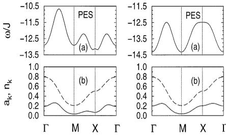
Fig. 1. Zero-temperature photoemission (PES) spectra in the main directions of the 2D BZ for  $U = 12t$  ( $J = t/3$ ): (a) QP dispersion and (b) momentum distribution  $n_k$  (dashed line) and QP weight  $a_k$  (full line); the special points as in Ref. [1]. Left panels:  $t' = -0.28t$ ,  $t'' = 0.18t$ ; right panels:  $t' = t'' = 0$ .
