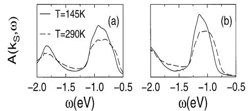
Fig. 3. Spectral function (1) at finite temperature for  $\mathbf{k}_S = (\pi/2, \pi/2)$ , with  $t = 375$  meV,  $U = 12t$ , and: (a)  $t' = -0.28t$ ,  $t'' = 0.18t$ ; (b)  $t' = t'' = 0$ . The broadening is fully due to the finite temperature.
