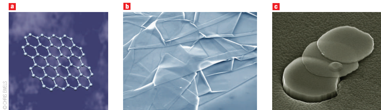
Figure 2 The structure of graphene. a , In graphene, each carbon atom is bonded to three other carbon atoms to form a two-dimensional honeycomb structure that displays a variety of novel electronic properties. b , c , Scanning electron micrographs showing a single graphene sheet ( b ) and thicker layers of graphite ( c ).
